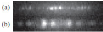
Figure 5. TOF images in a deep lattice and in magnetic traps with frequencies (a) 80 Hz and (b) 200 Hz. The speckles vary from shot to shot, and are due to interference during TOF of pancake BECs from different lattice wells.
